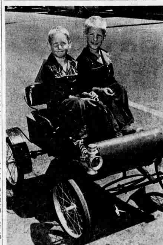
A MINIATURE 1903 Oldsmobile, built completely to scale, furnished the transportation for Ralph, left, and Ted Eccles in Saturday's Kiddie Parade here. The car, powered with a gasoline lawn mower engine, was constructed by the lads' father, Julian Eccles.
