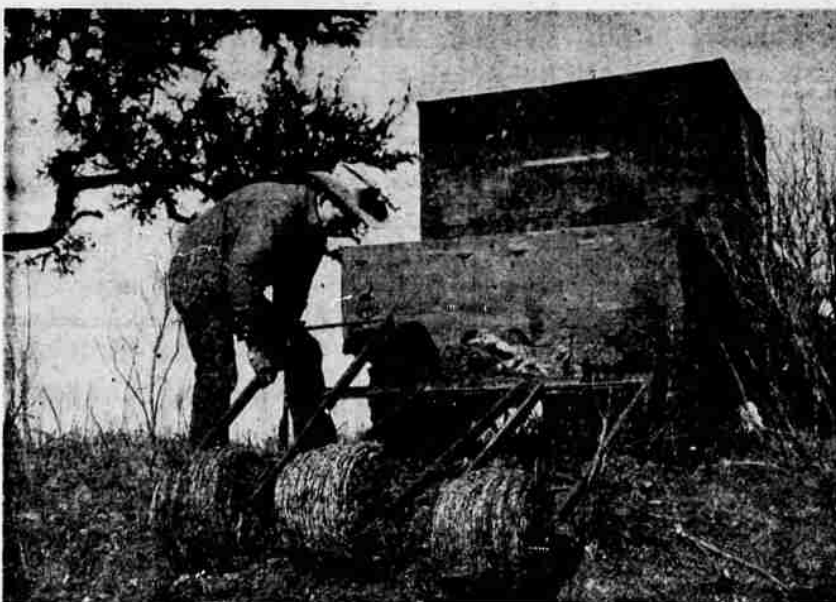
THIS NEWLY developed wire layer puts down three tightly pulled wires at the same time and is reported to halve the time normally required for fence work. The equipment, known as the Tumbleweed multiple wire layer, was recently invented by Dayton Hyde at the Yamsey Ranch near Chiloquin and is now on the market. Please see accompanying story for full details.
