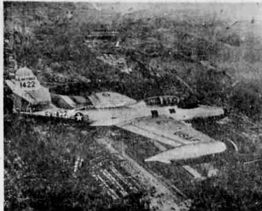
THE F-89D SCORPION is an Air Force interceptor type aircraft which carries a crew of two. Powered by an Allison J-35-3 turbojet engine...
