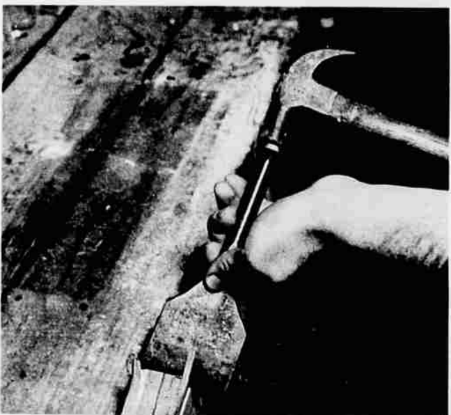
This is the proper way to hold chisel; if hammer slips, it will strike padded palm, not fragile bone.
