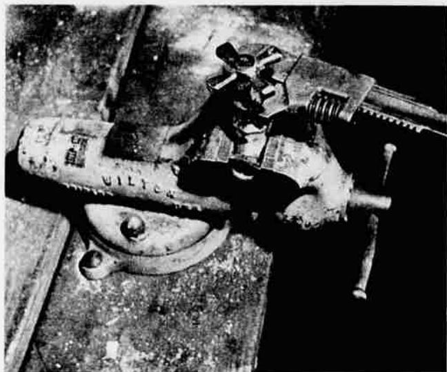
When working with wrench, operate it toward you; then, if it slips, you won't crash into work bench.
