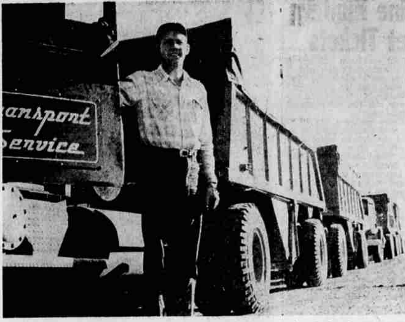
DIATOMITE shipments left Fort Rock recently for the Great Lakes Carbon Company refinery near Terrebonne. Harry Hutton, driver for Transport Service of Portland, is shown standing beside the hopper-bottom dump rigs as they were ready to roll. Four hundred tons will be hauled in the initial contract on a trial basis. The material is relatively light in weight, running about 1,200 pounds to the yard as mined. It is processed and used for filtering in many industries, notably in petroleum refining. — Photo by Parks.
