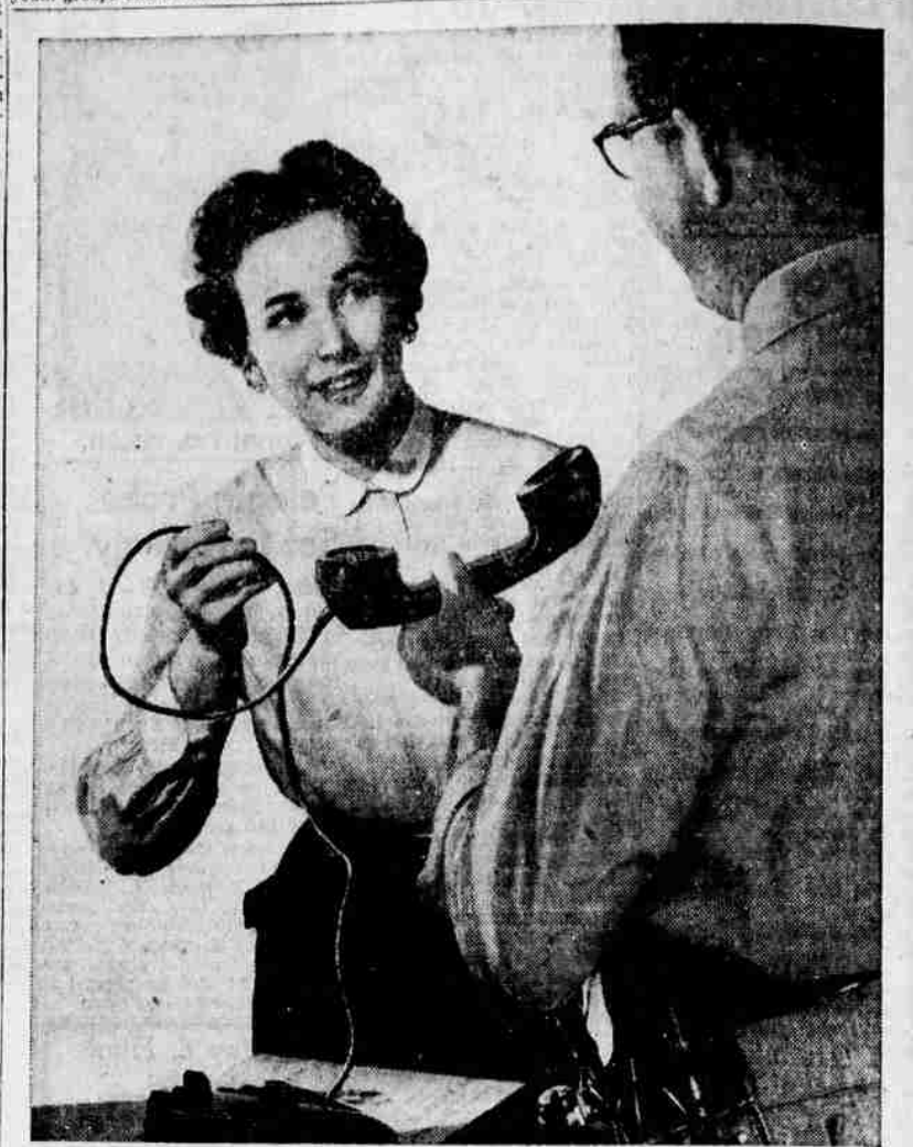
Rubber-covered telephone cord can really take it. The part of your telephone that gets the hardest wear is the cord. That's why telephone people now cover phone cords with synthetic rubber. This covering outlasts the cotton type by several years. Naturally, this helps keep telephones in good working order for even longer periods of time. It's another of the things that help us provide good, dependable service... service you can count on whenever you need it. The men and women of Pacific Telephone work to make your telephone more useful every day.
