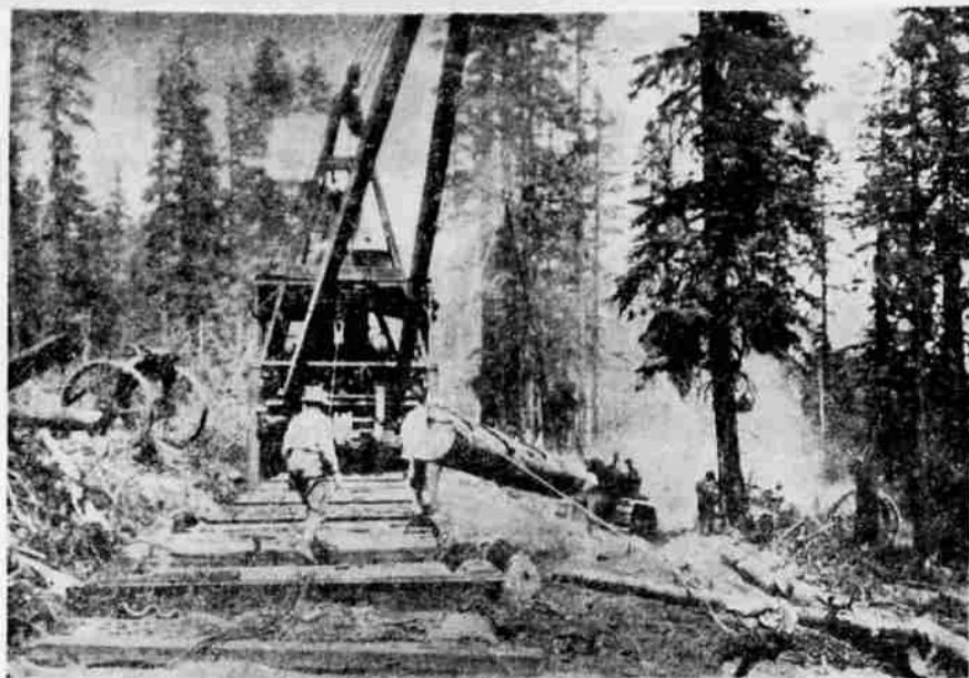
THIS CREW FROM THE BIG LAKES BOX COMPANY is shown loading logging flat cars for the trip to the sawmill. The site of this loading crew, photographed in the 1920's, was not recorded. The "hooker", lower left, had one of the hardest jobs in the logging camp. — Photo from A. J. Vaye collection, courtesy of A. D. Collier.
