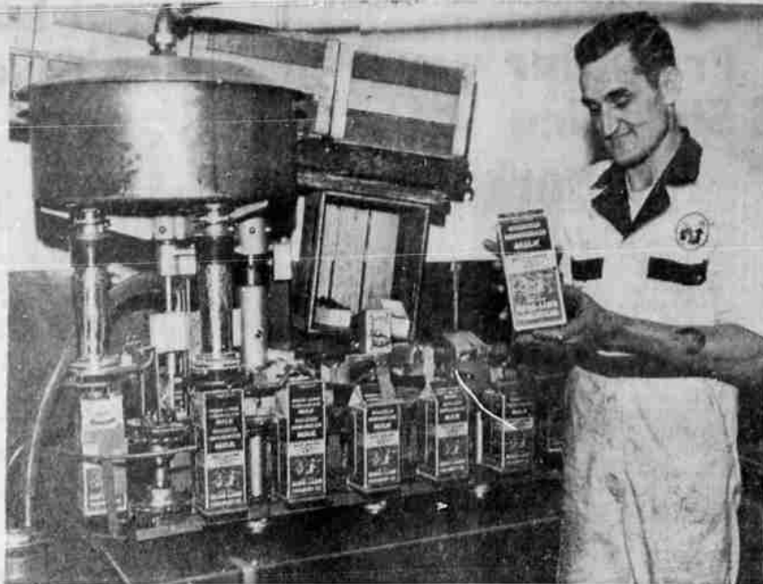
MEDO-LAND CREAMERY COMPANY is now supplying the local market with milk in half-gallon size containers. Charles Butler holds one of the new size containers just filled and sealed by the new half-gallon filler installed last week at the creamery. The capacity of the machine is 720 cartons per hour, according to Walter T. (Bud) Franklin, Medo-Land's Klamath Falls manager.
