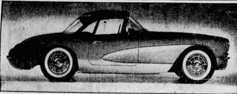
Chevrolet adds another chapter to its pioneering achievements with a new Corvette in the sport car field. Among principal features are a power-actuated fabric top lift and a removable solid top, which like the body is built of reinforced glass fiber plastic. The car has been completely restyled and offers either a manual or Powerglide transmission coupled to a V8 engine of 235 horsepower. In appearance the latest Corvette may be readily distinguished from previous models. Rear fenders sweep downward and the sides of the body carry a sculptured depression. Exterior color choices list black, green, copper, red, blue and white, with the cockpit color-keyed in beige or red.
