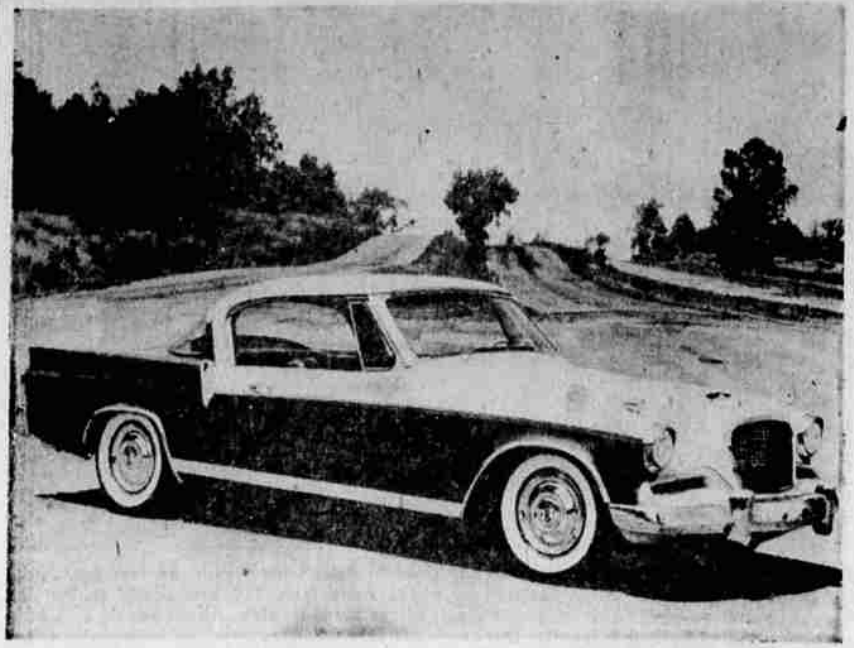
THE GOLDEN HAWK, top model in Studebaker's special line of sports-type models, is the highest powered car in the low-price class for 1956. It has a 275-horsepower 352-cubic inch V-8 engine, developing 380 foot pounds of torque at 2800 revolutions per minute. It has four-barrel carburetion and a compression ratio of 9.5-1. The 5-passenger model is 17 feet long, six feet wide, less than five feet high, in sharp contrast with Studebaker's new standard models which have moved to a big design. Three other sports-type cars round out the special line, first full line to be introduced by an American auto manufacturer: the Sky Hawk, with a 210-horsepower V8 engine; Power Hawk with 170-horsepower V8; and the Flight Hawk with a 6-cylinder in-line economy engine of 101-horsepower. The Golden Hawk will have the Studebaker-Packard Ultramatic transmission as optional equipment, the other three models using the new Studebaker Flightomatic transmission. Instrument panel on the Golden Hawk will have a race car inspired dashboard panel which includes a tachometer and vacuum gauge. Equipment includes new safety-fin brakes which minimize fade after successive stops, 12-volt battery electrical system, full range of optional power equipment, noise deadening headlinings, and padded instrument panel. Special safety features include optional seat belts, tubeless tires, and safety door latches. It is sold by Juckland Sales and Service.
