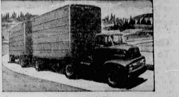
NEW CARRYING CAPACITY throughout the line. New Ford F-500, "1 1/2-tonner," for example, has new 15,000-lb. GVW—an increase of 1,000 lbs.! New higher-capacity tubeless tires standard equipment on all models!
