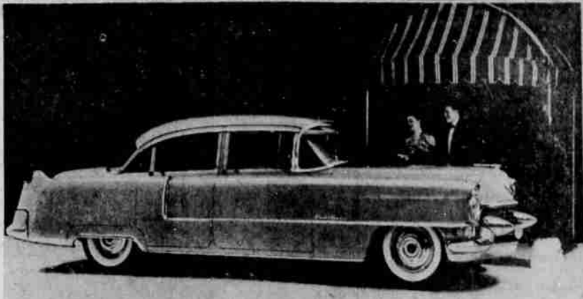
AMONG THE MANY distinguishing styling features of the 1955 Cadillac series 62 four-door sedan are: Florentine curve rear window styling similar to the series 62 coupe and coupe de ville; integral rear fenders, and a redesigned bright chrome and stainless steel cellular grille with grille extensions. The 1955 Cadillac series 62 sedan is powered by a 250 horsepower high compression V-8 Cadillac engine. The new Cadillac is now on display at the Dick B. Miller Company, 710 Klamath Avenue, in Klamath Falls.
