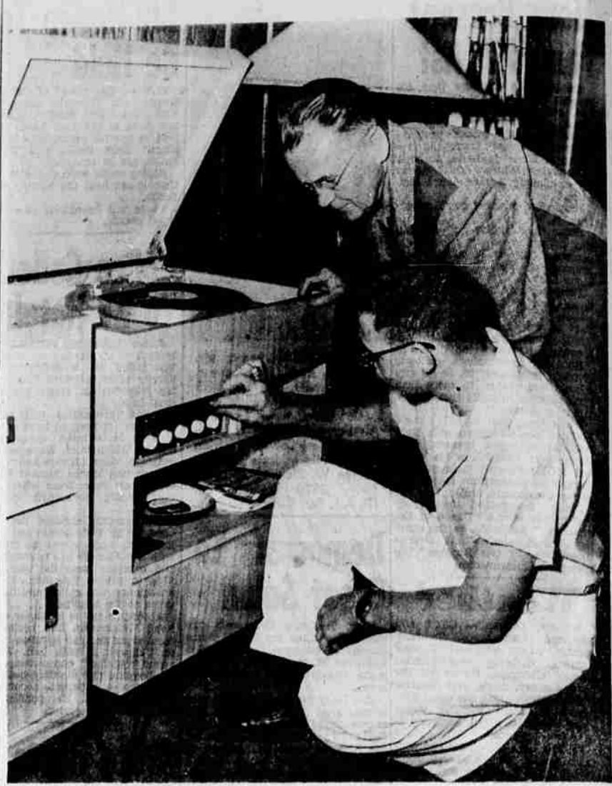
NEW HIGH FIDELITY SOUND SET assembled by Sam Thompson, (kneeling). Components of set include Fairchild pickups, Livingston arm, Cook preamplifier-equalizer, Craftsman and Heathkit amplifiers, 15 inch Electrovoice and Jensen speakers mounted in separate bass reflex cabinets. Lewis Stanley, president of the Klamath Falls Amateur Radio Society looks on as final tests are made. The set is believed to be the only one of its kind between Portland and Palo Alto.
