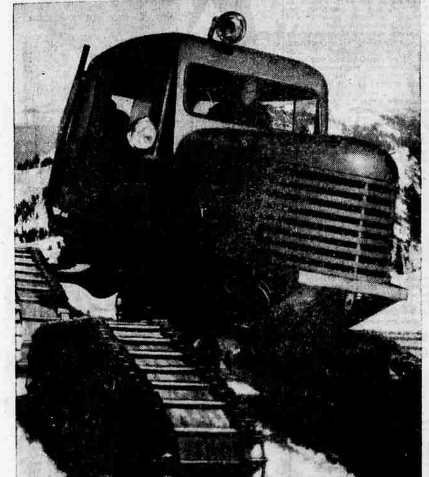
Sno-Cats stalk trouble in the mountains. High in the snow country of the Pacific West, winter blizzards are fierce and frequent. Here motorized Sno-Cats help telephone crews roll out fast to stop trouble before it can interrupt service. The powerful "Cats" carry 6 to 8 men comfortably, cruise over the snow and ice at speeds up to 25 miles an hour. Using these vehicles instead of skis or snowshoes, our mountain crews patrol vast areas faster. They can spot such potential troublemakers as leaning poles, broken branches, wires buried in towering snow drifts. By saving valuable time and helping prevent trouble, the Sno-Cat helps us cut costs, hold down the price of telephone service to you. Pacific Telephone works to make your telephone a bigger value every day.
