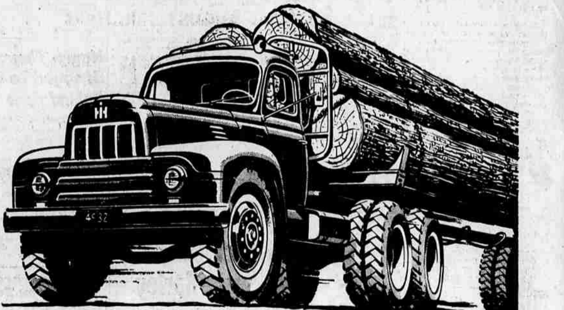
23 new 6-wheel models. GVW ratings, 22,000 to 90,000 lbs. Choice of gasoline or LPG fuel systems. Diesel engines available for models with GVW ratings of 30,000 lbs. and over.
