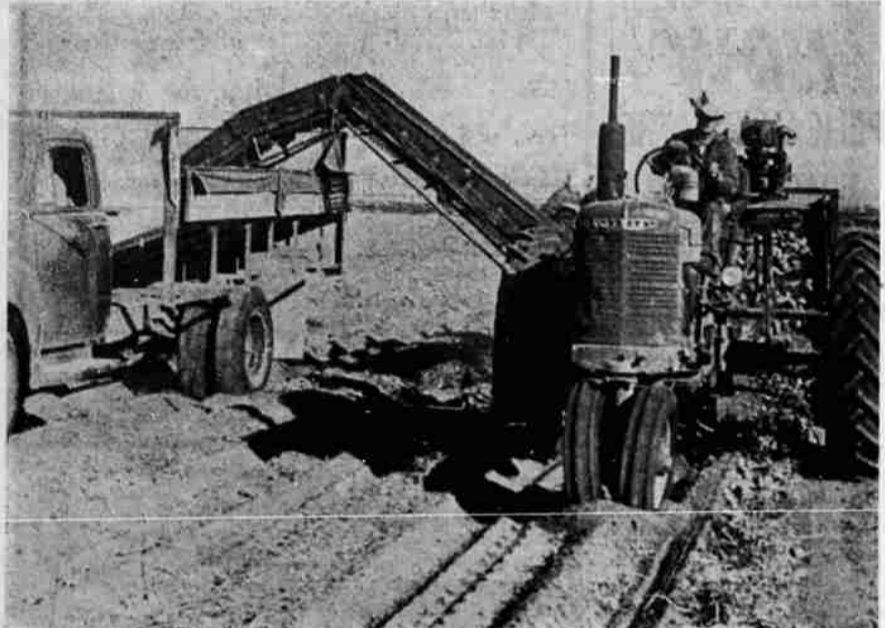
A BEAN MANUFACTURING CO. BULKER of the type used by the Osborne Brothers at their Macdoel place. This particular two-row bulker is digging in sand soil.
