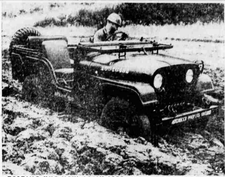
TESTING THE NEW ARMY JEEP — Mud up to hubcaps can't stop the Army's new jeep during debut at Aberdeen, Md. Proving Ground. The engine can be replaced in 14 minutes.
