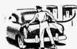
THE OLD WAY—Gas filler cap on fender...unhandy to reach from far side...unsightly.
