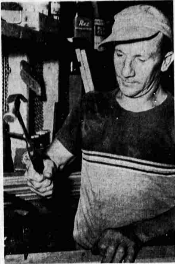
AXEL FLOREN , local contractor and house builder, has received patent No. 2,603,260 for a shock absorber hammer. The type he is shown demonstrating here has a spring handle beneath the grip wrapping.
