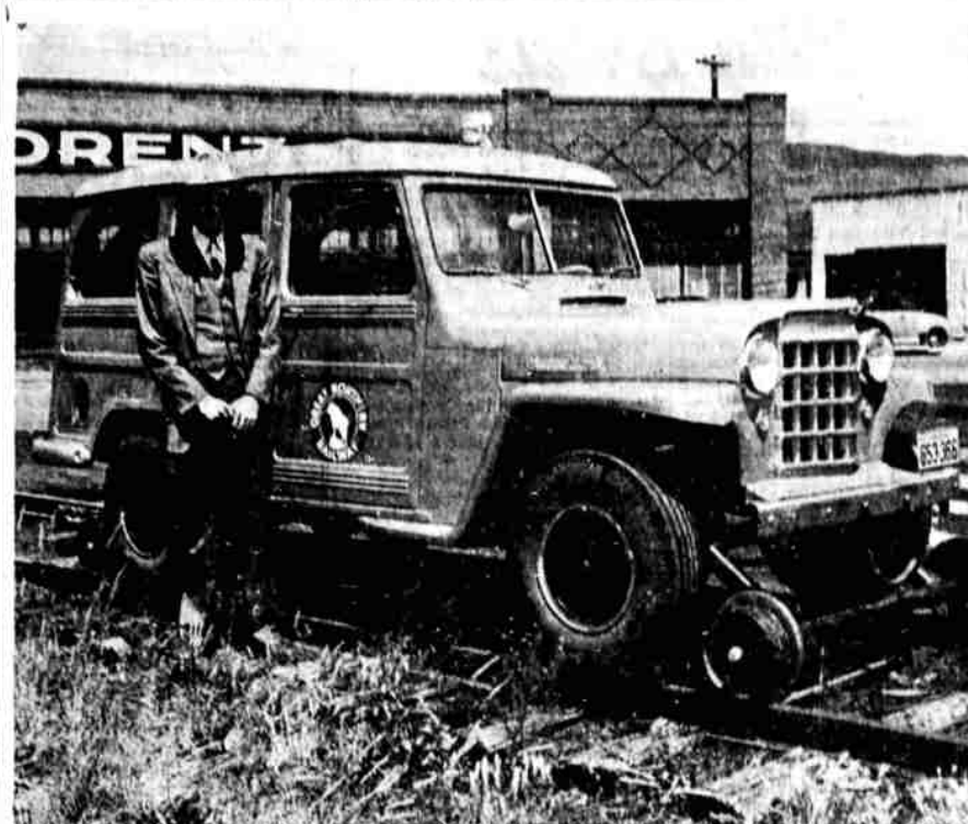
INNOVATION on "speeded" type transportation used in railroading is this Hy-Rail car recently put into operation here by the Great Northern Railroad. Built from a Jeep station wagon by the Fairmont Motor Co., Fairmont, Minn., it can ride both on rail and on highways, merely by lowering or retracting "landing-gear" guide wheels. The guides seldom touch the rail, merely guide the wheels of the car with its flanges. The gear is hydraulically operated. On the highway the car has jeep-speed, and on rail it can hit about 50 miles per hour. The tires are eight-ply, and operate the car by traction. Eugene F. Oviatt, Klamath superintendent, poses by the car—one of the first to be introduced into the Northwest. It will be used to check rails, ride out spurs, and various other duties.
