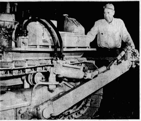
GAINING POPULARITY this season is this Caterpillar No. 42 tool bar, exhibited by the Crater Lake Machinery Co. Here Otto Ellis looks over the tool bar, which can be used for cultivating, bordering, chiseling, disk ridging, listing, furrowing, subsoiling and numerous other things. Hydraulically operated, the bar should make farming easier.
