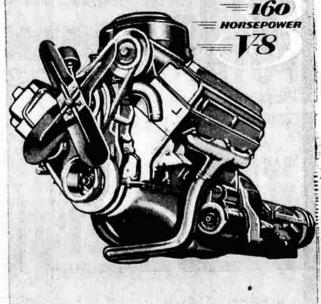
FIRE DOME has famous dome-shaped combustion chambers with centralized spark plugs . . . the engine design that gets more power from every drop of gas. This new De Soto will be the most talked about car of 1952. See it TODAY!
