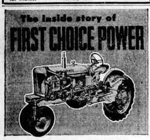
Look at the inside of the WD Tractor-see what makes it today's first choice in tractor power. PLENTY OF FULL for heavy jobs such as plowing with 3 full-size bottoms. Traction booster puts full engine
