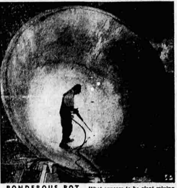
PONDEROUS POT —What appears to be giant mixing bowl is actually world's largest cast steel cinder pot, one of 27 being built by U. S. Steel for hot slag in open hearth shop.
