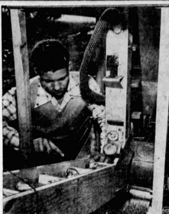
INVENTS "BULB SNATCHER" —Johnny C. Williams of Fayette, Ala., looks over the ingenious machine that he designed to process gladiolus bulbs. The "bulb snatcher" counts the bulbs, sprays them with DDT and grades them for market. The 16-year-old farm boy is hailed by his neighbors as an electrical wizard because of many similar labor-saving devices he has built. Johnny is one of six winners in Westinghouse's 4-H "Better Methods" contest.
