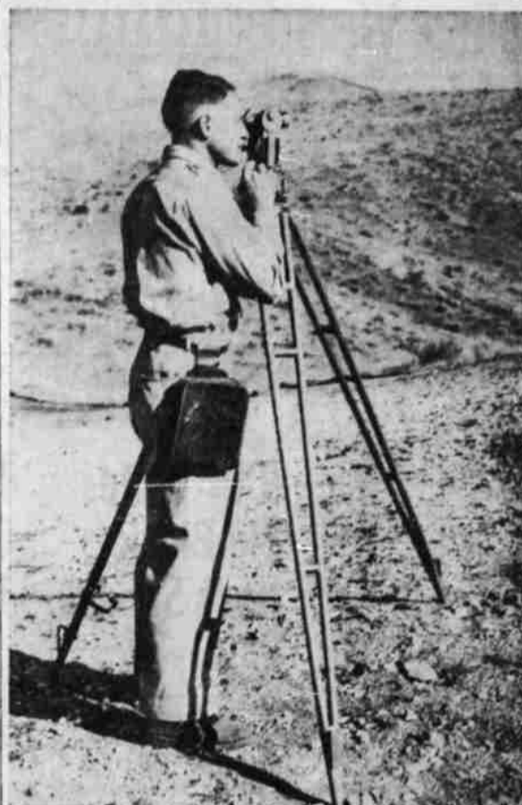
SIGHTIN' OUT—Project Engineer C. V. Eckhardt takes a sight through a theodolite—a high-precision transit—while taking shots on triangulation points. Eckhardt is in charge of a survey being conducted by the U. S. geological survey, which is charting more than 1800 square miles of Modoc and Siskiyou county land in California. The survey is finding control points which are used in laying out aerial maps of the area. The project is slated to carry on until winter weather moves in.
