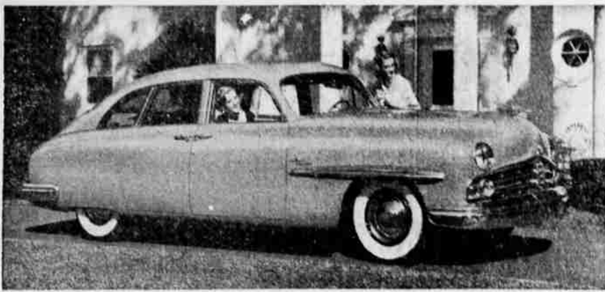
Streamlined elegance and maximum comfort are achieved in the 1949 Lincoln Cosmopolitan Town Sedan. Completely new from roof to road, it features a new 152-horsepower 8-cylinder V-type engine and completely new suspension, chassis and body.
