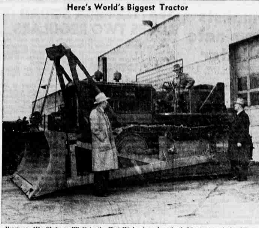
Here's an Allis Chalmers HD-19 in the West-Hitchcock yard on South 7th street, ready for delivery to Pat Ivory of Ivory Pine Lumber company, shown at right looking over his new behemoth, R. McNaabb is at the controls and Phil Hitchcock at left. The HD-19 is billed as the world's largest, most powerful tractor. It weighs 40,000 pounds, has 163 net engine horsepower, and a hydraulic torque converter drive.
