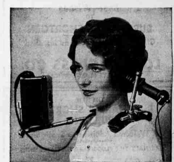
1. This gadget was the latest thing in headsets when grandmother was a girl. Matter of fact, it was the first headset in general use back in 1880. It weighed more than six pounds. It's a museum piece now, of course. Headset styles changed. They grew lighter, more comfortable, more efficient.
