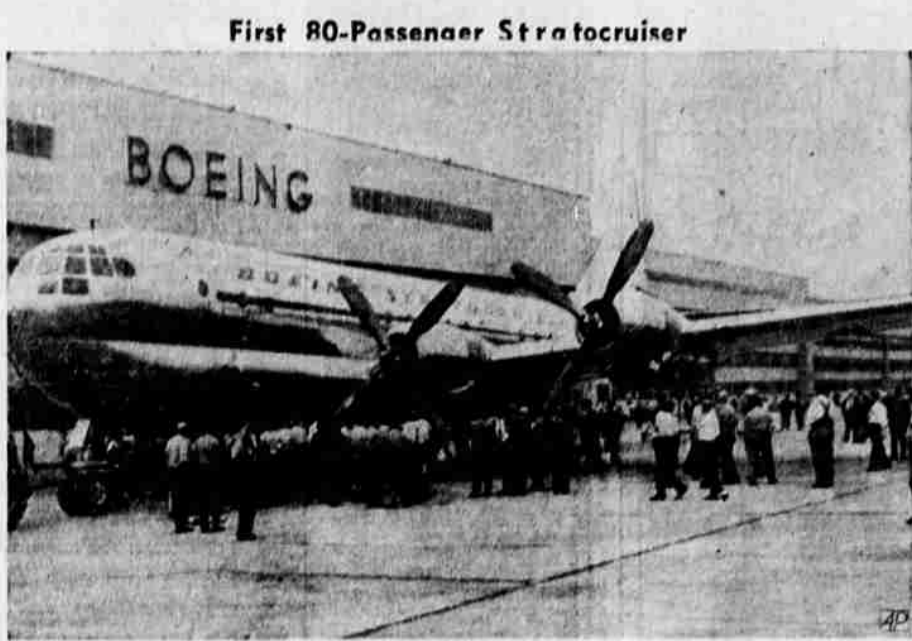
A crowd gathers at Seattle to inspect the first 67½-ton strato-cruiser as it rolls from the Boeing plant. Luxurious, 340-mile-an-hour double-deckers of this type are scheduled to go into service on airlines late this year.
