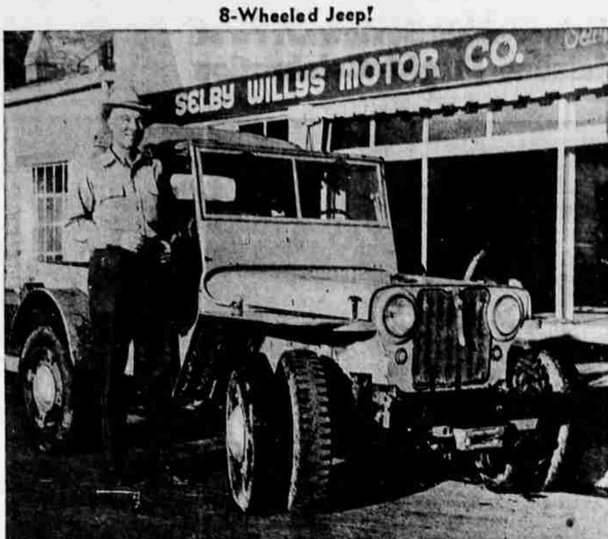
Shown above is A. F. McQuiston of the D & M ranch at Fort Klamath and his 1946 Willys jeep which is equipped with dual tires on both front and rear. The jeep, which was purchased from Selby Willys here, had the extra four wheels installed in order to give it greater flotation and to prevent ruts in meadows on the ranch. It is used in irrigating, transporting personnel, and general farm work and, according to McQuiston, "can operate where tractors or even horses cannot get."
