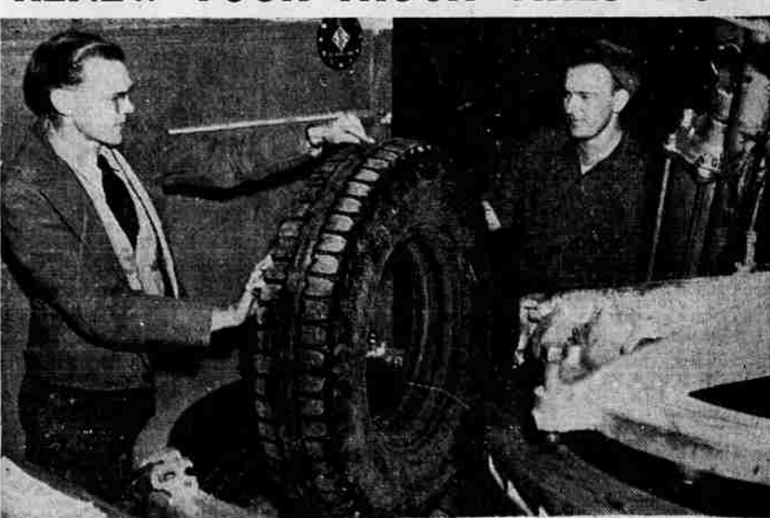
Ross Johnston, Balsiger tire department manager, and Merle Wickline examine a "Stop-Start" truck recap just out of the mold. These recaps cost less than half the price of new tires and will equal new tire mileage.
