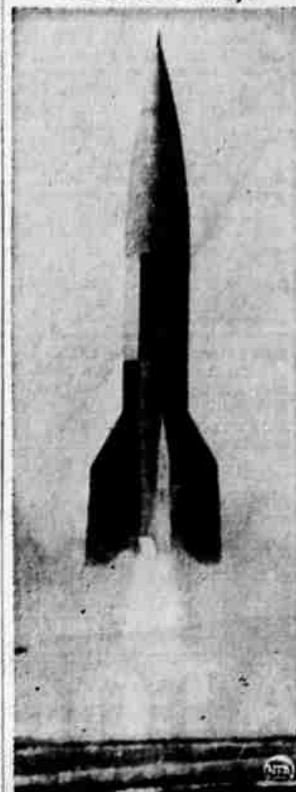
Belching flame and smoke amid a cloud of dust, a German V-2 rocket rises from its platform at White Sands proving grounds, N. M., where army ordnance is testing the deadly German weapon. Testing of this huge 46-foot, 28,000-pound missile, will allow scientists to study the stratosphere at an altitude of 100 miles.
