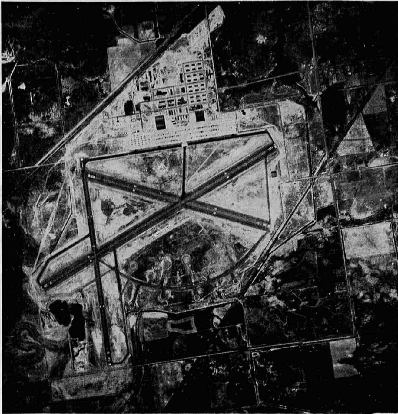
A vertical air view of the whole naval air station with the runway is pictured above. The long diagonal runway is nearly a mile and a half long and two others are almost a mile long. This view is taken from an altitude of 14,500 feet. —Official U. S. navy photo.
