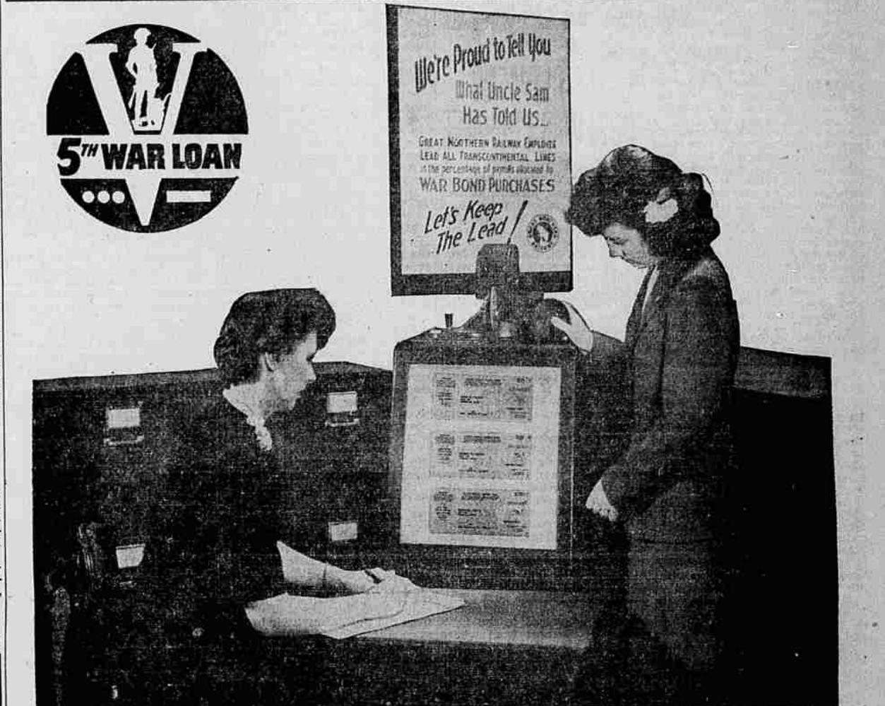
Issuance of War Bonds by the Great Northern necessitates full-time employment of 22 persons at company expense. Records of bonds issued are photographed on 16 mm. film. The machine above enlarges film records, enabling speedy check on inquiries.
