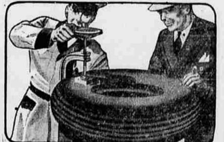
**WE PATCH SMALL BREAKS...** Injuries to the sidewall of a tire are often signs of a blowout on the way. A "spot" repair is made and vulcanized to the rest of the tire. Tread cuts and other causes of trouble should also be repaired before it's too late.
