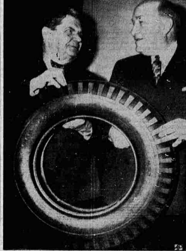
Rubber Administrator William M. Jeffers (right), shows Senator Raymond E. Willis (left) what Jeffers termed the nation's first all synthetic heavy duty truck tire. The tire was built by Goodyear with butadiene produced from alcohol manufactured at an Institute, W. Va., plant which utilizes grains.
