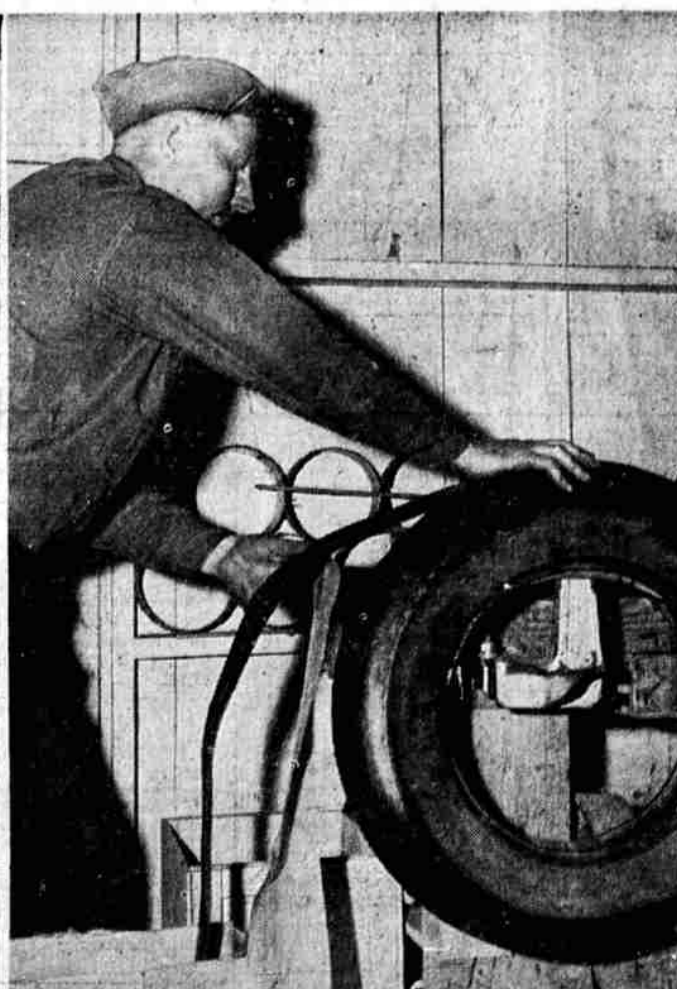
4 "Camelback"—rubber re-capping—is then placed on cemented surface. In continuous strips, camelback is blue seal, highest grade material, gives the motorist mileage equal to new tire. Guy Wilson is shown applying it to old rubber.
