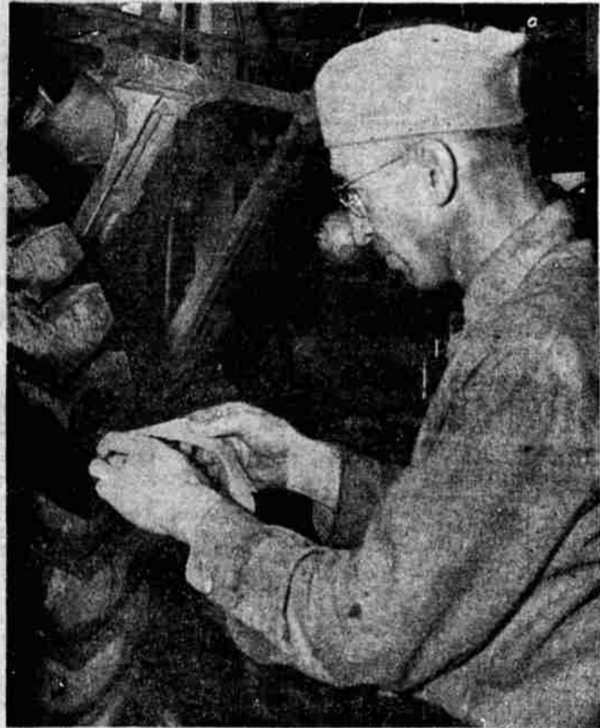
1 First step in re-capping process, if tire needs section filler, is raw rubber plug. Like an infected tooth, tire cavity is drilled out and layers of rubber inserted. Cement and cohesive action make it stick. Earl Young shows how it's done.
