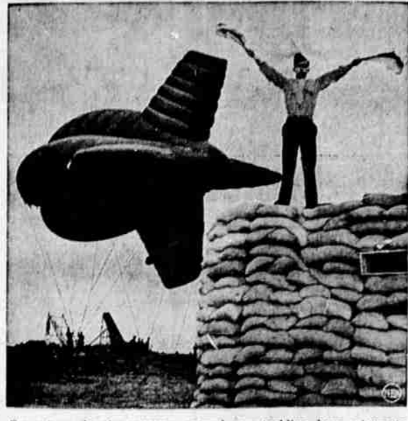
Semaphore signaller messages ground crew bedding down a barrage balloon, much-used defender against dive bombers, at Marine Corps Parris Island, S. C., base. Wig-wagger stands on hut housing winch which controls height of gas bag.
