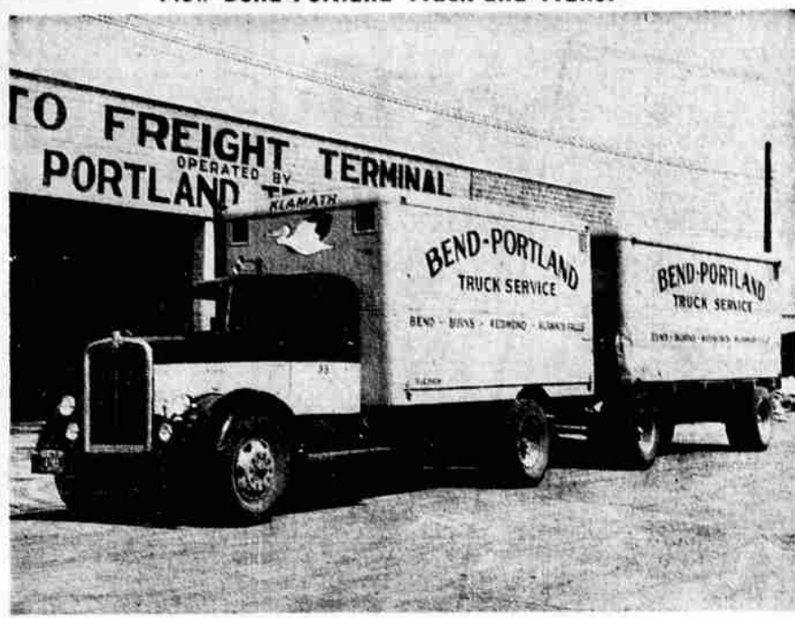
Here's a brand new unit recently purchased by the Bend-Portland Truck line for daily round trip use between Klamath Falls and Portland. It's a new Kenworth diesel with a supercharged 200-horsepower motor and 14-ton capacity. The truck, known as the Klamath Pelican, is painted the standard Bend-Portland orange and black colors.
