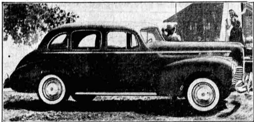
All new 1941 Hudson models are lower, longer, and more graceful in "tailor-made" styling. The new body styling is the sweep of the new rear deck design with the accompanying new design of rear quarter windows and a roof panel. This new styling in combination with a 2-inch reduction in overall body height and an increase in body length of 5 1/2 inches, enhances the smooth, harmonious flow of body lines. The model shown above is the Commodore Eight Touring Sedan on 121-inch wheelbase and powered with 128 horsepower engine. Featured in all 1941 Hudsons is a new style development called Symphonic Styling which offers a choice of interior color combinations that harmonize with exterior colors.
