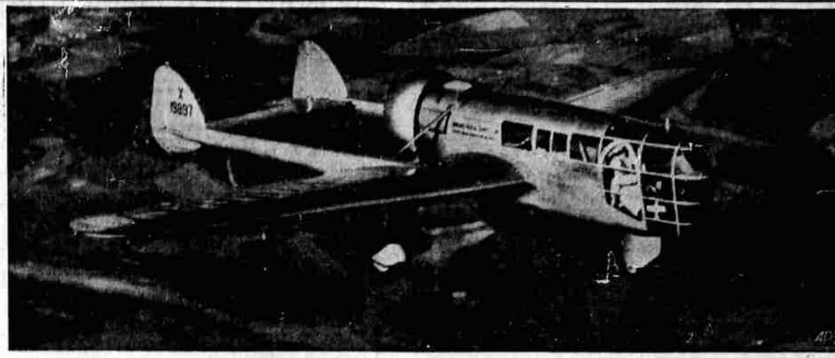
ONE WAY TO SURVEY —Designed so that pilot, sitting in front, has unobstructed view, this pusher-type Abrams plane is used for high altitude photographic surveys. It climbs 20,000 feet in 20 minutes; tricycle undercarriage insures safer operation.
