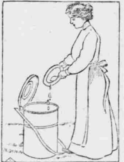
LID RAISES BY FOOT PRESSURE. refuse it is not necessary to touch it with the hands, a pressure of the toe answering all purposes. Extensions of the handle acting as levers engage pins in a steel strap riveted to the top of the can, so that by pressure of the foot the hinged lid is easily lifted. A loop at the back of the lid serves as a stop to keep it from swinging beyond a perpendicular position and when the pressure is released permits it to close by gravity.
