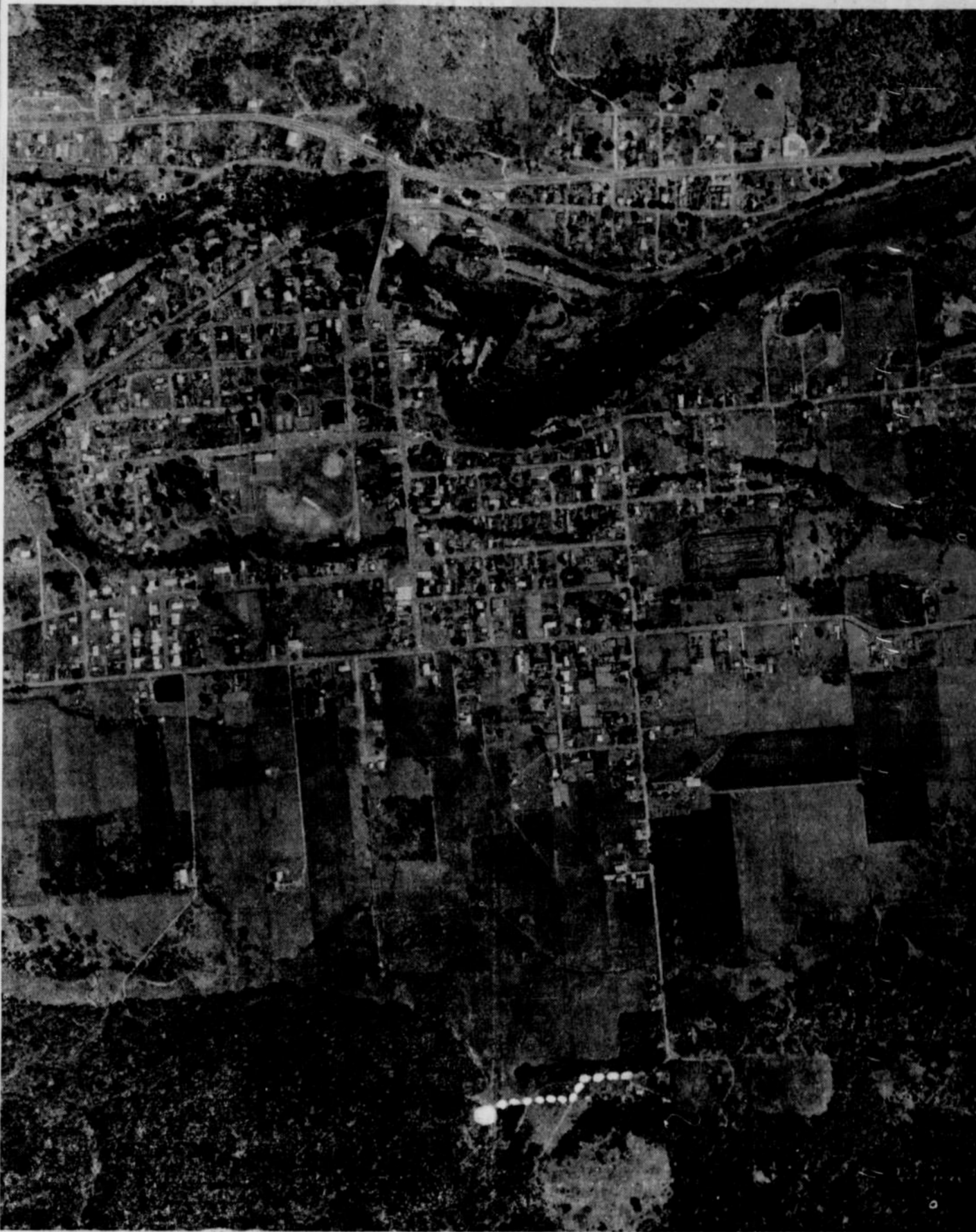
Aerial photo of Mill City shows route of new road (dotted line) being constructed to the site of a new Pacific Power & Light Company water reservoir indicated by white dot at bottom center of photo. The 250,000-gallon tank will augment existing facilities in Mill City to provide water service to the rapidly growing southwest portion of the town.
