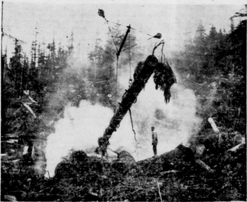
MEHAMA—Loading a log truck in the woods is done by a loading donkey. Above, the "crotch line" method is being used to load logs at the Vincent Keller logging operations at the foot of House Mountain in the North Santiam area.
