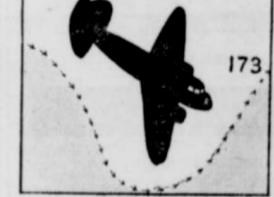
Captain Eddie Rickenbacker, noted flier, says there's no such thing as an air pocket or partial vacuum in the sky, as plane passengers believe. There are only currents of air, some upward, some downward, depending on the winds, etc. The so-called air pocket is merely a descending air current of good solid air—the same that, if it were ascending, would be called a "bump." Plane passengers will have to revise their terminology, for talking of "air pockets" is only a sign of ignorance these days.
