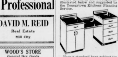
Here a standard base cabinet top is hung between two standard steel base cabinets at a level 30 to 31 inches above the floor. It is firmly supported on a wood strip secured to the wall and by bolts secured to the side panels of the cabinets. This forms an ideal kitchen desk,
