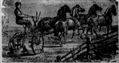
With Flexible Pole, Land Guage, and Leveling Lever. It is raised out of the ground by a brake arrangement, and can be handled by a boy old enough to drive the team.
