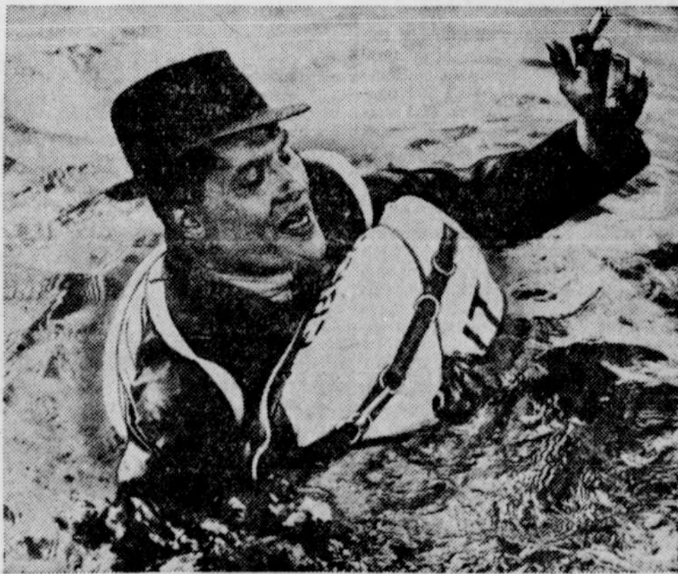
This adaptable smoker is demonstrating a new safety chair used by the Imperial Airways flying boats. The apparatus consists of special cushions, built on the float-on-air principle, which form the upholstery of the passenger seats and can quickly be transformed into a life-belt. It weighs only five pounds and can support a weight up to 230 pounds in the water.
