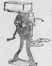
Will fit in any location to suit the owner. The crank is put on the most convenient side and a pulley for Engineor Motor power attached opposite
