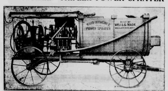
Manufactured in the northwest to meet the conditions, strongly built, plenty of power and displacement, and will do your spraying thoroughly and cheaply. Capacity sufficient to maintain four lines of hose, with two nozdes each, operates two guns, uniform pre-sure evenly maintained at any point. The Triplex Pump guaranteed to test 600 pounds working pressure. Send for catalog, and see demonstration
